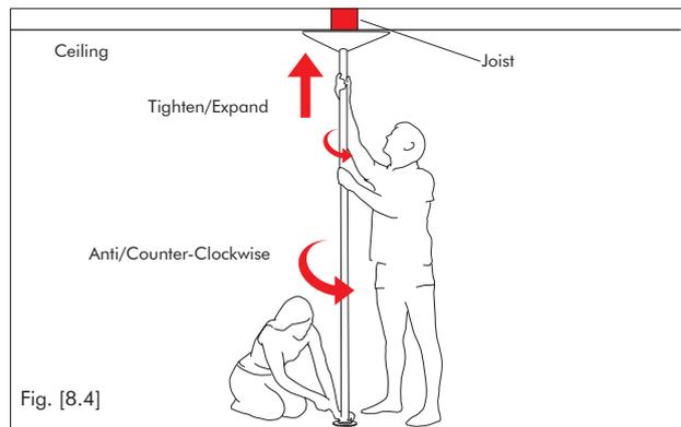
4. Pole Expansion: Rotating the main pole tube from left to the right (Anti/Counter-Clockwise) will Expand/Tighten the Pole. Rotating the pole tube from right to the left (Clockwise) will Shorten/Loosen the Pole.
