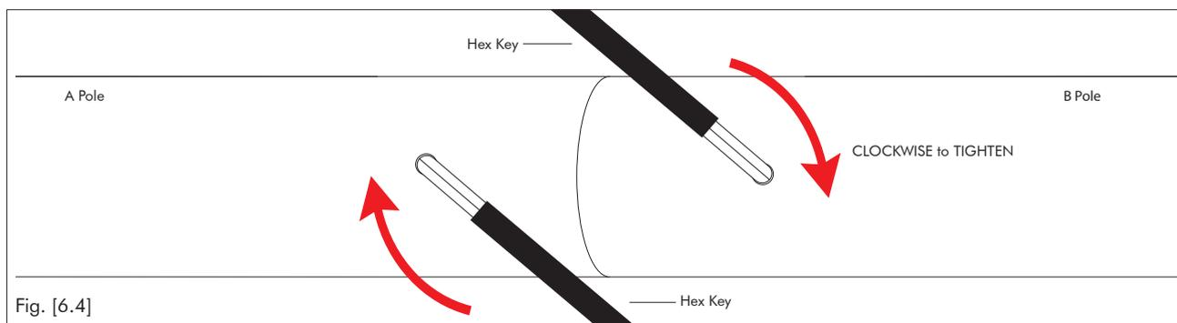
4. It is important to tighten the screws progressively – alternating between the screws, tightening Clockwise. This will ensure the pressure is equalised within the pole tubes.
