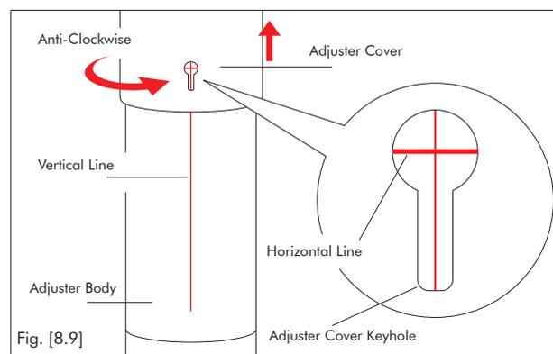
10. When expanding/unwinding the pole Anti/Counter-clockwise, the adjuster cover will rise. If a horizontal line on the adjuster is exposed in the keyhole – this indicates that the adjuster is close to 100mm. It is at 100mm when the line is below the adjuster cover. Consider buying an extension from our website [www.xpole.com](http://www.xpole.com)
