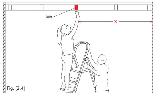
3. To find a Joist above your ceiling, tap across the ceiling with your knuckle until a solid sound is heard – this will be the Joist. If you keep tapping across the ceiling the sound will become hollow – the space between the Joists.
