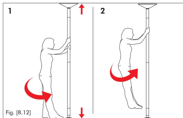
12. Once the pole is tight, rotate the pole till the Adjuster Cover Keyhole is in alignment with the vertical line on the Adjuster. This will ensure that the screws are on the flats. Now tighten the 3 Adjuster Locking Hex Screws tightly with a 5mm Hex Key to lock the A-Pole.
