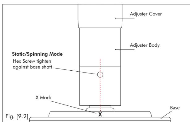
1. To change the pole mode from static to spinning – undo the 2 x Static/Spin Hex screws at the bottom of the pole, until they are flush with the pole - **DO NOT REMOVE COMPLETELY** – the pole will now spin freely.
