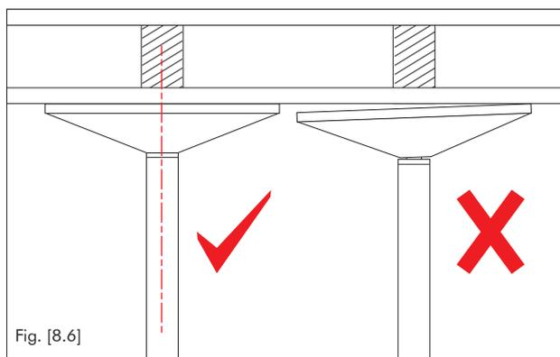
7. It is critical that the Upper Dome is flat against the ceiling/Joist. DO NOT expand the adjuster further until the upper dome is flat against the ceiling/Joist. If the Upper Dome is not flat, the plate could rotate, and slip or damage the ceiling.
