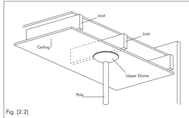
1. The XPERT POLE should be installed in the most secure location possible, like under a solid ceiling – if you do not have a solid ceiling, you will have to locate a 'Joist' or 'girder' to install the upper dome against.
