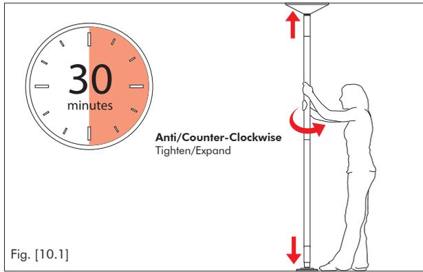
1. Because the XPERT pole uses pressure to remain in position. The pole tightness should be checked regularly during use, ideally every 30 minutes.
