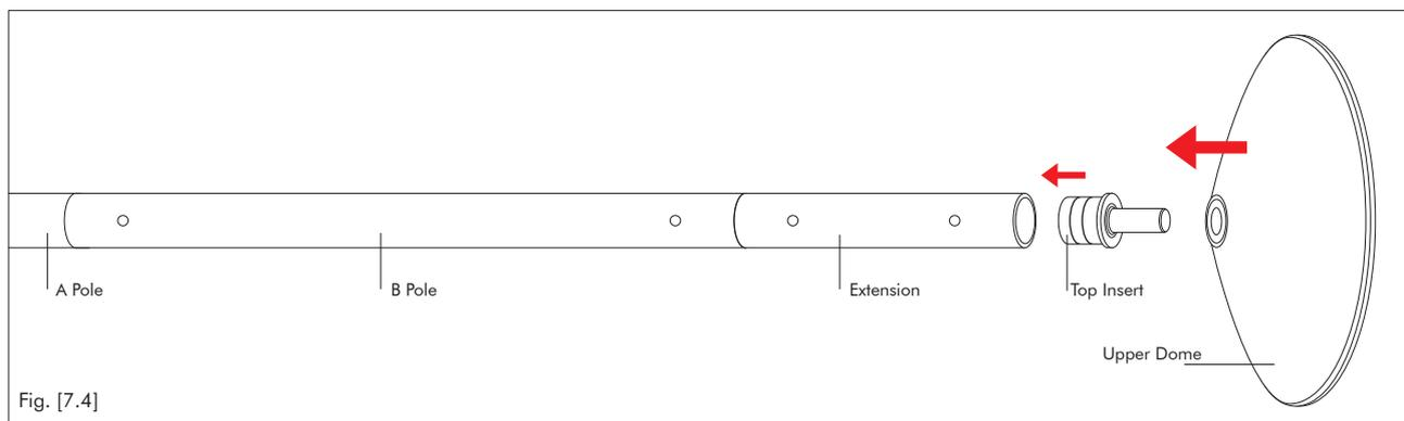
1. Once the A-Pole and B-Pole (and any additional extensions) are connected, insert the Top Insert into the B-Pole or last extension used then slide the upper dome onto the top insert.
