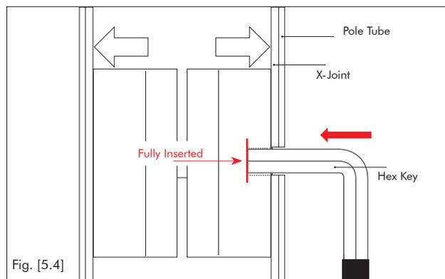
3. The X-Joint features a special mechanism which expands/contracts to lock/loosen the pole tubes together. Please test this prior to assembly.
