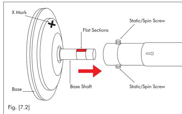
2. Make sure the 2 x Static/Spin screws are fully loosened using the 5mm Hex Key. **DO NOT** completely remove the screws. Slide the base shaft into the A-Pole. The two screws need to be in line with the X's on the base to ensure they are screwed onto the flat sections.
