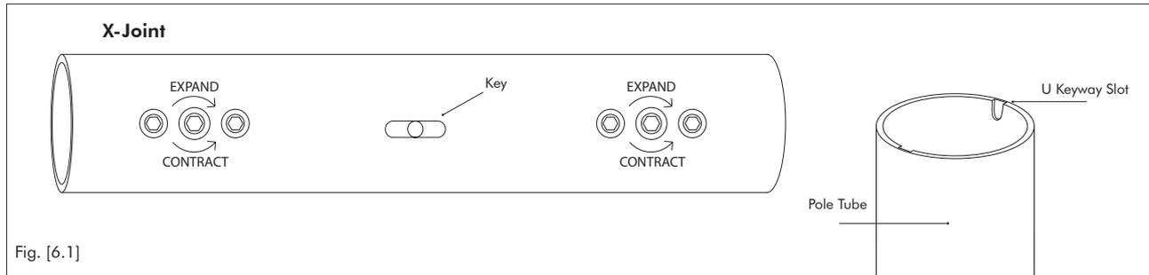
1. At the centre of the X-Joint are 2 x Keys. These Keys slide into the corresponding U Keyway slots in the pole tube.
