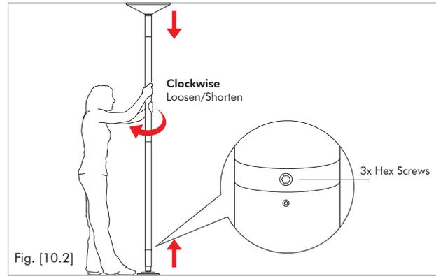
2. To take down the pole, undo the 3 x Hex Adjuster Locking Screws (DO NOT completely remove the screws). Then turn the pole clockwise to contract/release the pole. Once the pole has been removed from its position, the Upper Dome & Base can be removed.
