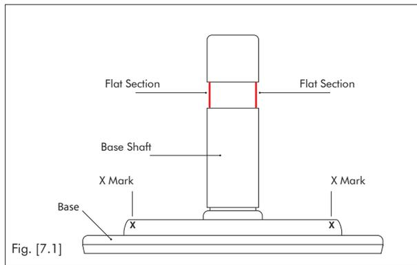
1. The 2 x flat sections are where the hex screws will locate to stop the pole from spinning. Note the 2 x flat sections on the base shaft, and ensure these are in line with the X's on the base.
