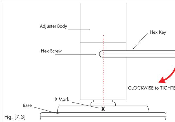
3. Once the A-Pole is on the shaft – align both the Static/Spin screws with the 'X-Marks' on the base and tighten the 2 screws.
