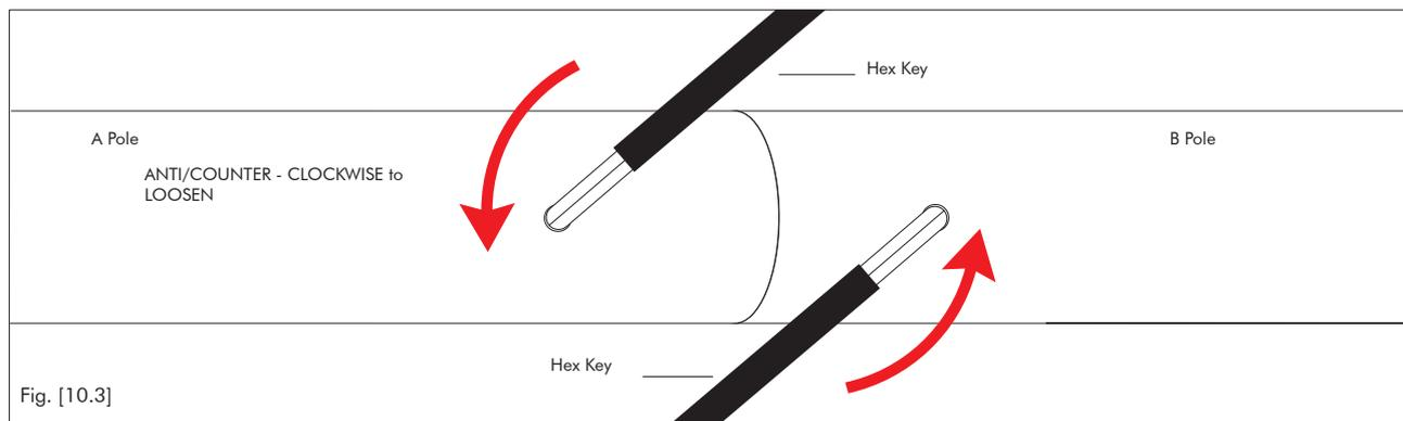
3. Lay the pole tubes on the floor and undo the X-Joints to disassemble the XPERT. To undo the X-Joint – turn both Hex Screws **Anti/Counter Clockwise** – undo screws until there is pressure against the key.
