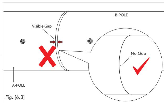
2. Insert a 200mm X-Joint into the A-Pole ensuring the keys locate into the U Slots and the expansion screws line up with the holes on the pole tubes. Next attach the B-Pole to the A-Pole with the X-Joint ensuring the Keys engage with the U Keyway Slots.
